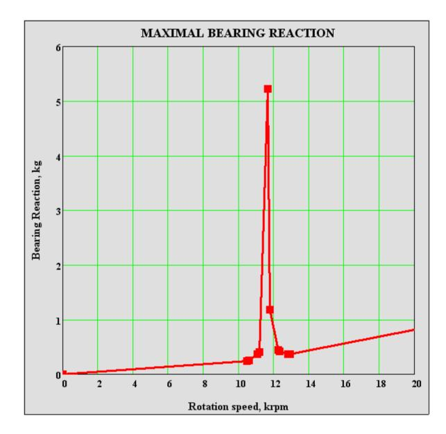
The simulation was performed using MSC\Nastran for Windows. In this software package, it is not possible to perform a rotor dynamics analysis. Therefore, the bearing reactions were calculated by formula. The formulae used for the calculation of the bearing reactions are:
