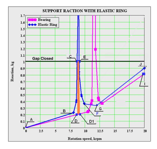
Magnitude of the Maximal Reaction as Rotation speed Function:
