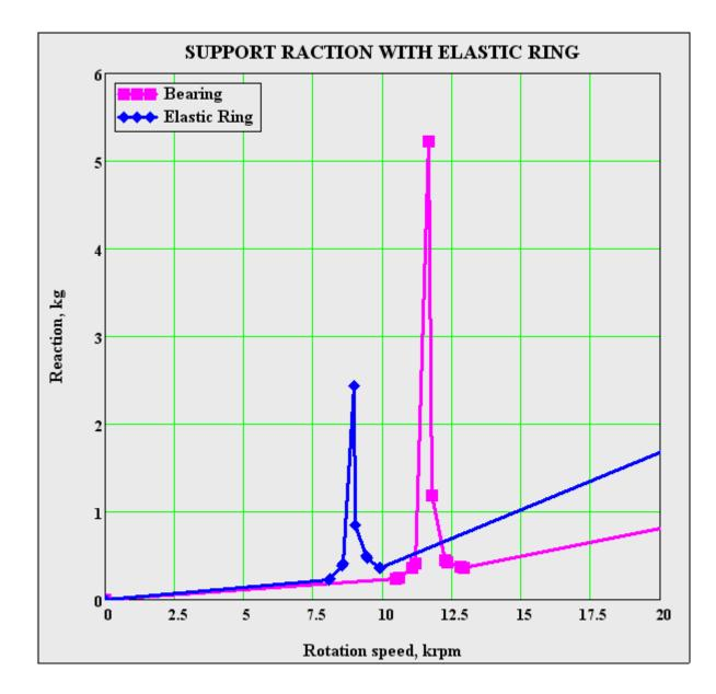
After we placed an elastic ring around the bearing, the stiffness of the support became nonlinear.
