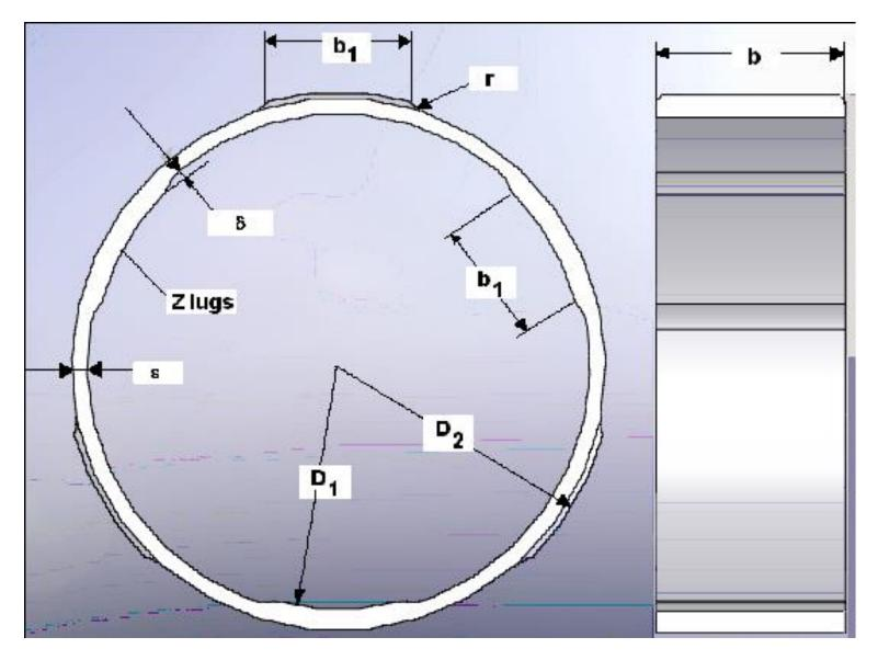
With the geometry of the ring know, its stiffness can be calculated.
