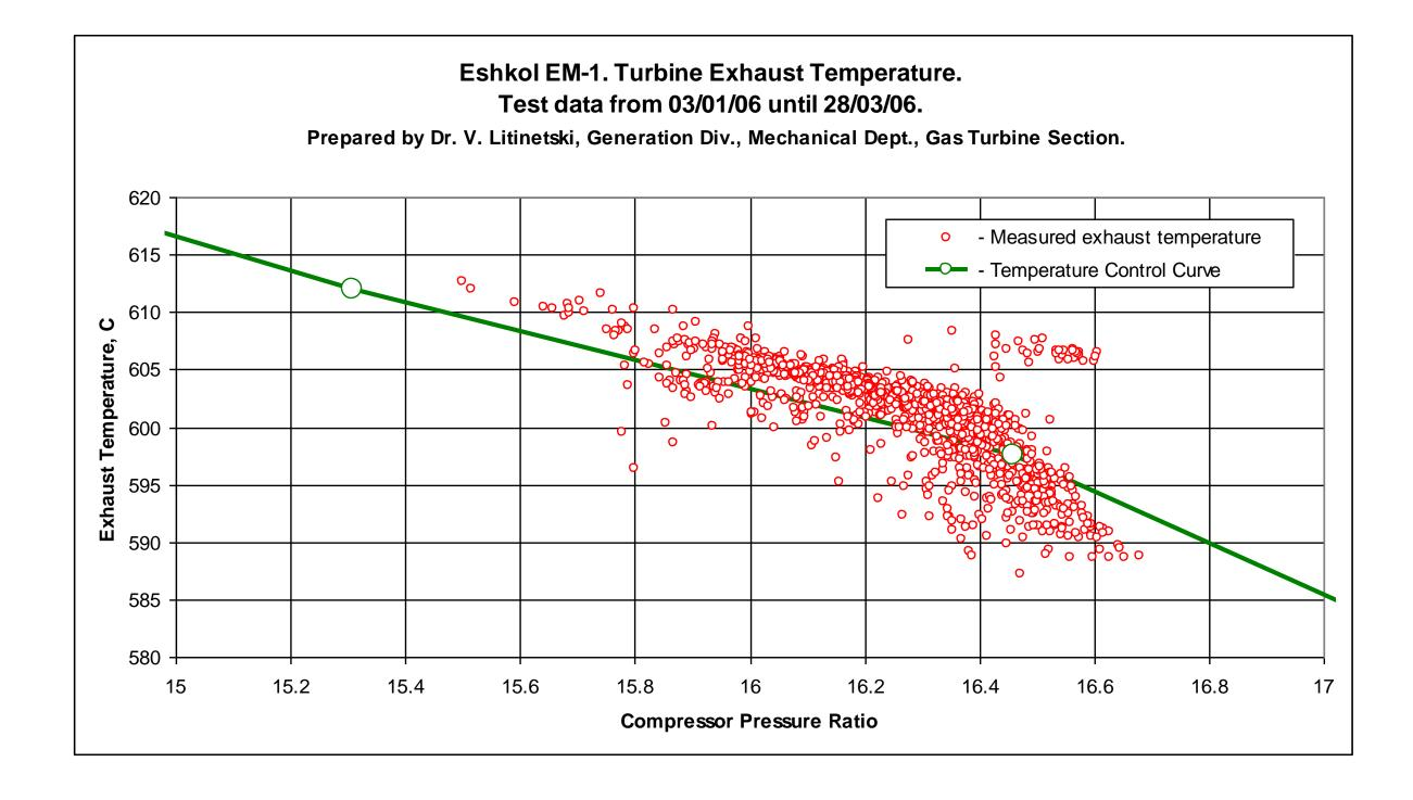
Thorough analysis of the data revealed an error in the control system software, namely, an incorrect definition of so called Temperature Control Curve, which is an important element of the turbine load control, fuel efficiency and protection (Figure below).
