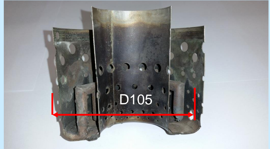
Combustor with 6 vaporizers, small jet engine
