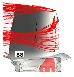
Secondary flow vortices disrupt the cooling effectiveness from the film cooling. This effect is mainly seen on the suction side.
