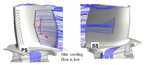
Last row of cooling flows on the pressure side seem to have some ingestion.
