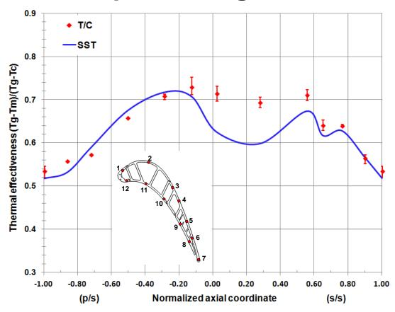
CHT model with SST with transition does an adequate job predicting metal temperatures except on a few points on the suction side.
