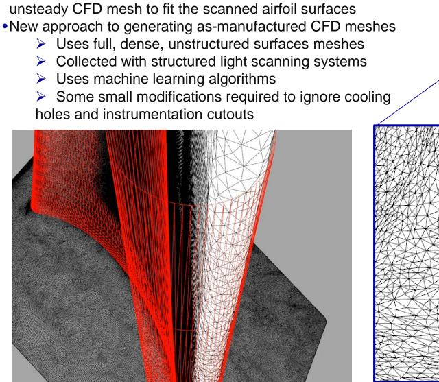
MORPH algorithm used to alter the as-designed "blueprint"
