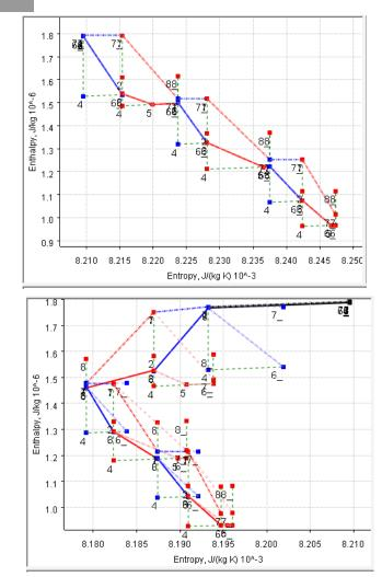
Enthalpy-Entropy Diagram of uncooled & cooled turbine
