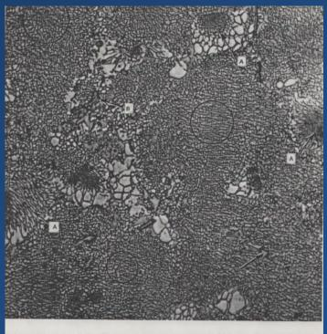
WA 1455 Material After Attaining Metal Temperature of Less than 2000°F (1094°C) Exhibiting Typical Uniform Array of Matrix Gamma Prime Precipitate (Circled Areas), Gamma-Gamma Prime Eutectic Islands (A), RD PRACTICES and MC-type Carbides (B) Figure 1 (1000X)
