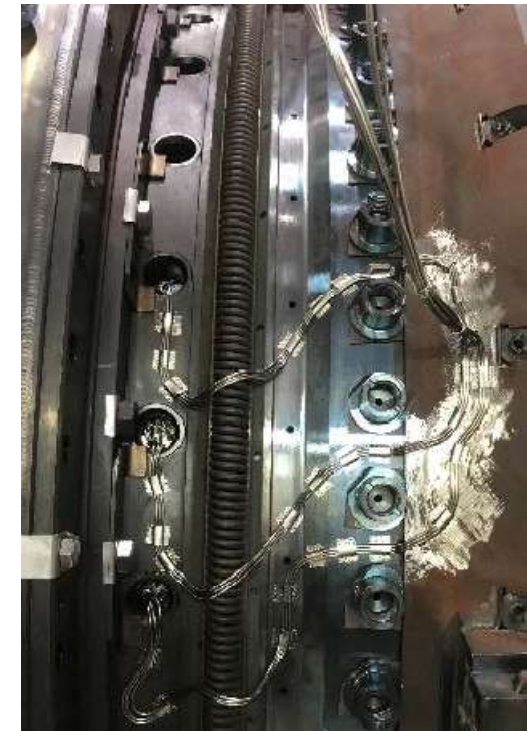
AM GV Thermocouples lead out Instrumentation on the Customer Engine
