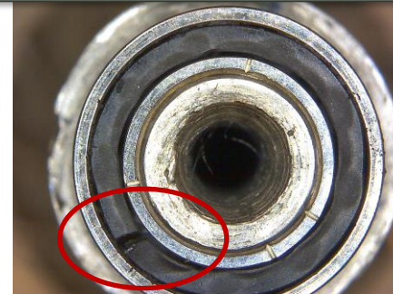
Broken bearing cage due to vibrations
