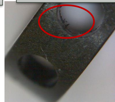
Cage wear (insufficient lubrication)
