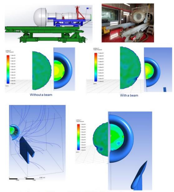
Aerodynamic profile beam cut (NACA0030, 30° inclination angle)
